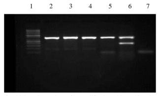
**Fig. 4.** Gel electrophoresis of multiplex PCR products after amplification with specific primers for *bla*<sub>VIM</sub> gene (391 bp)
