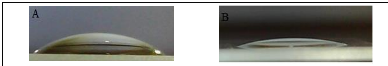
Fig. 4. A water droplet on A) the non-treated surface that produced 30° angle and B) 150 s helium-treated surface that produced a 10° angle
