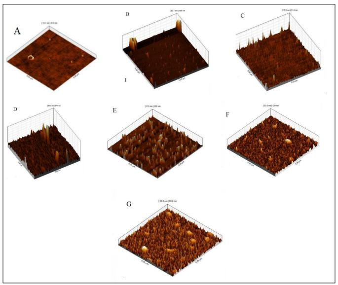
**Fig. 3.** (A) 3D AFM images of  $5\mu m \times 5\mu m$  of untreated sample; B) 3D AFM images of  $5\mu m \times 5\mu m$  of surfaces treated with Helium plasma for 150 s (B), 220 s (C) and 300 s (D); 3D AFM images of  $5\mu m \times 5\mu m$  of surfaces treated with Helium plasma covered with immobilized lysostaphin protein for 150 s (E), F (220 s), and 300 s (G)
